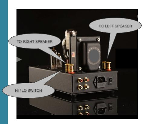
This amplifier can operate speakers as low as 2 ohms, and as high as 16 ohms and everything in-between. No harm can come to the amplifier if the speaker jacks are shorted together.
