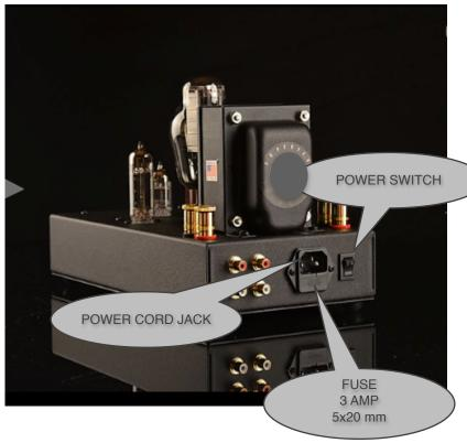
Make sure power cord is fully inserted into power cord jack. A loose cord can cause reliability issues with the tubes and potentially the amplifier itself.
