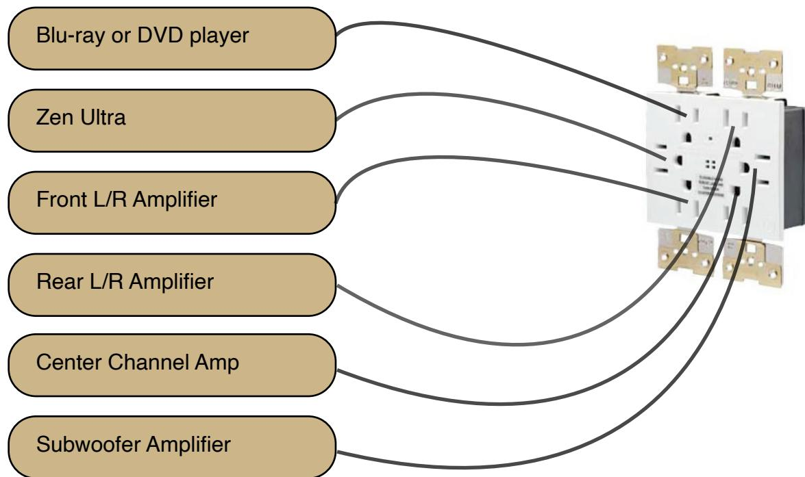
The example above is ideal. If you have additional sources, you'll want to have two of these types of receptacles. The idea is to keep the receptacles as close together as possible and with the least number of wiring connections. This creates a nearly ideal "single point ground". Most tube amplifiers that are 50 watts or less draw only an amp or two and source components even less. This sample would estimate a 10 amp draw that would be OK for a single 15 amp circuit breaker.
