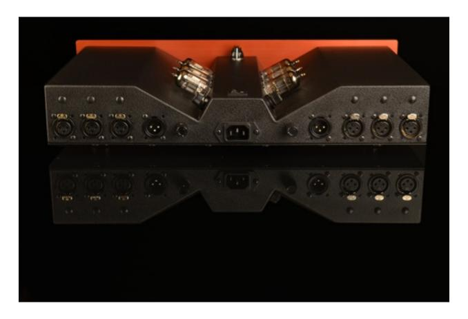
ZTPRE is designed for the higher heater current requirements it's factory tube compliment of 6N1P-EB tubes. These are the smoothest and the warmest tubes available making use with digital sources particularly synergistic. Replacement tubes are always available from DECWARE.
