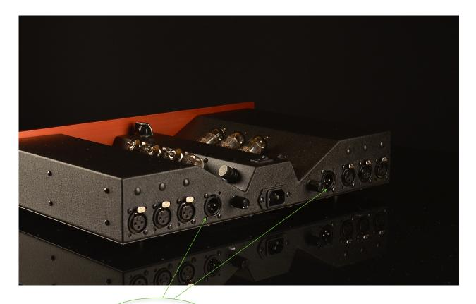
The ZTPRE has two XLR fully balanced outputs, one per channel that are directly connected to the output level controls previously discussed.
