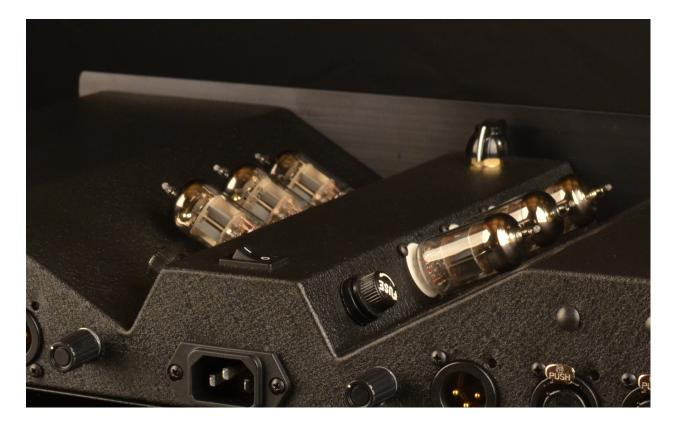
The three tubes of each channel have the heaters wired in series which means that ideally you want all three tubes to match. It definitely means that where the factory tube compliment of 6N1P-EB tubs are concerned, you either have to run all 6N1P-EB's or NONE at all. In other words, you can run 6922's, good strong 6DJ8's, or 7DJ8's. Some Russian 6N23P's may also work well so long as they are relatively matched.
