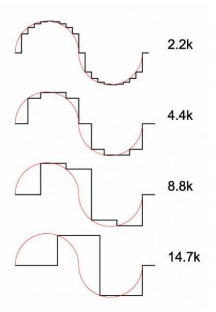
If you look at a digital approximation (black) of an analog wave (red) you can see that the right angles actually create minute increases in amplitude. Even after all the fancy algorithms of todays DSP DACS there still seems to be at minimum an echo of these hard points in the waveform.
