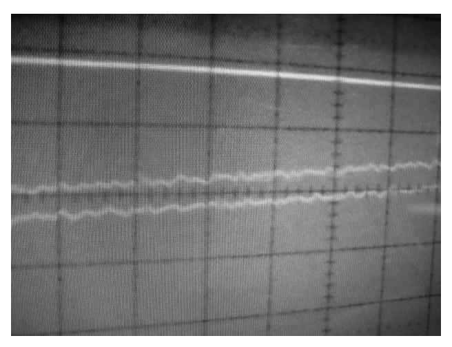
Waveform from analog function generator (top), vs. Waveform from an Apple iPod (bottom).
