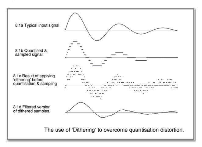
Quantization, dithering and filtering are all attempts to get a smooth continuous thread like analog. As you can see, filtering essentially glues all the dots back together and compresses them back into a fine line similar to the original input signal but with a rougher texture.
