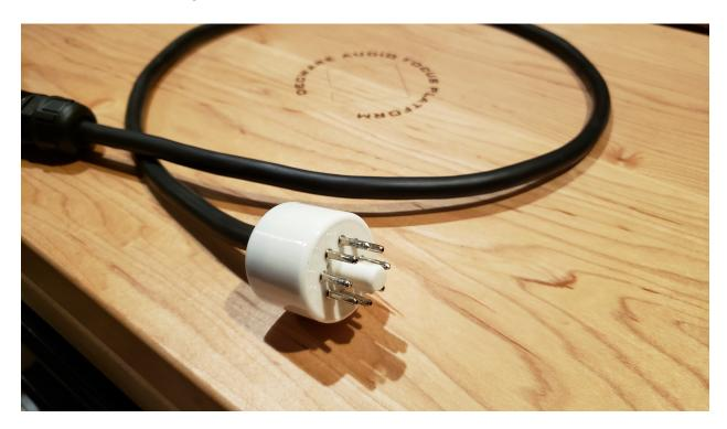
To install the cable, first connect it to the DynaGrid with the twist lock connector, and then to the component by inserting it exactly as you would a rectifier tube. Be sure both units are turned off before you begin.
