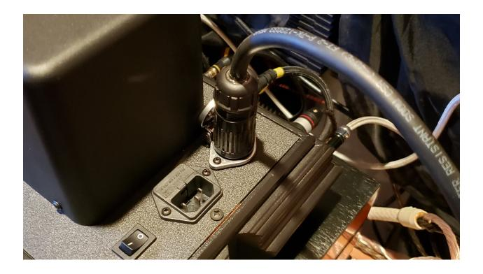
The DynaGrid Jr. has the high voltage interconnect cable jack located in the rear. The picture above shows the cable installed into the jack.
