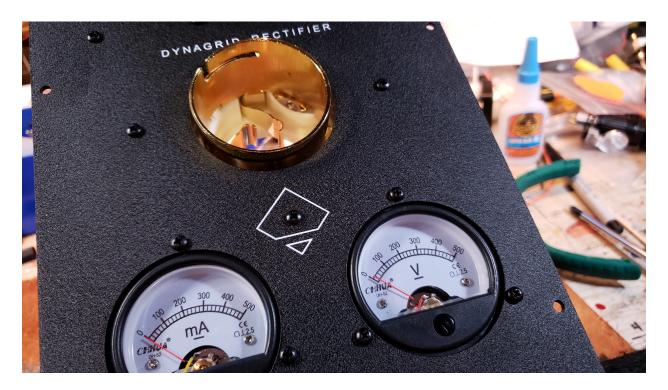
The DynaGrid Jr. has two meters on it. One is the voltage of your component and the other is how much current the component is drawing.
