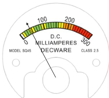
There are four switches below the meter that are laid out similar to the output tubes they represent. You may use one switch at a time to see the current draw of it's corresponding tube - or you may use two switches at a time - typically used to see the total current for a channel. And you can use all four switches at the same time to view the total current for all of the output tubes. This is a common use for the meter while the amplifier is playing.
