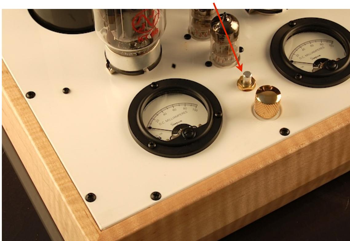
In the picture above you can see the meter on the left is for the KT88 output tube directly behind it. Same for the meter on the right. These meters show how many millamps of current are going through each output tube. Since this is a push pull amplifier, the objective is to get both tubes to draw the same amount of current so that they match. This gives the best performance and the most power.
